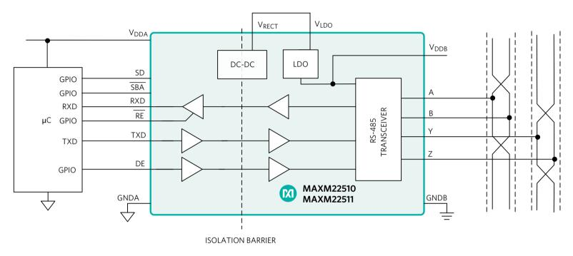
Figure 10. MAXM22511 Isolated RS-485 in Full-Duplex Configuration
