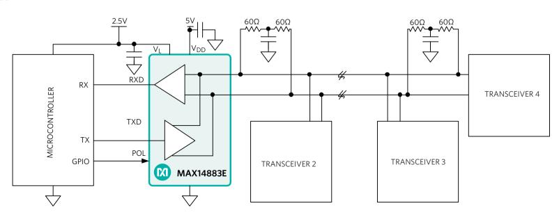
Figure 11. MAX14883E CAN Transceiver with Polarity Select
