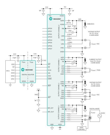
Figure 2. MAX22007 Configurable Analog Output demonstrating multi-mode application
