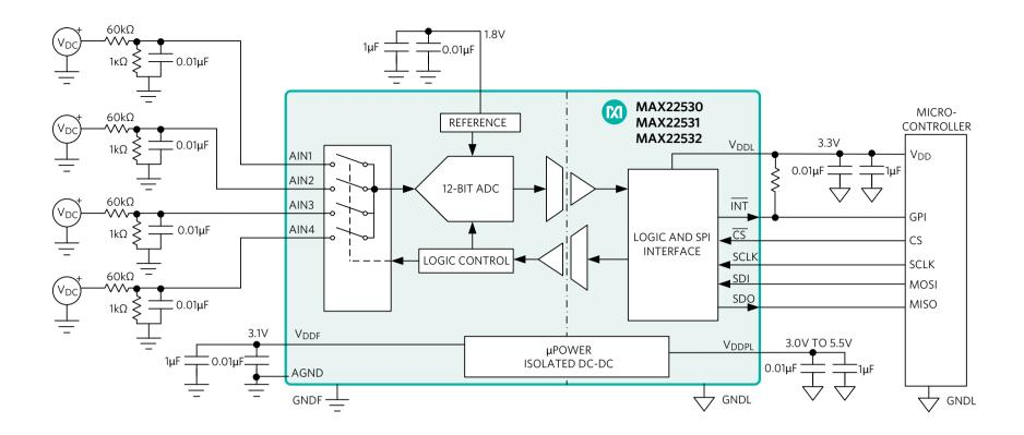
Figure 8. High DC Voltage Monitoring using MAX22530 Isolated ADC
