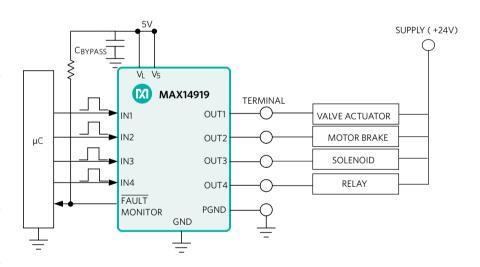
Figure 9. MAX14919 Quad Low-Side Switch
