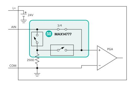
Figure 13. MAX14777 Quad BTR Switch Application Circuit
