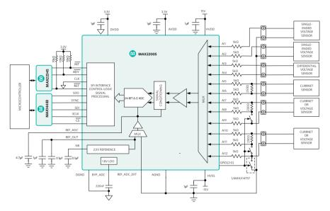
Figure 3. MAX22005 12-Channel Configurable Analog Input Application Circuit
