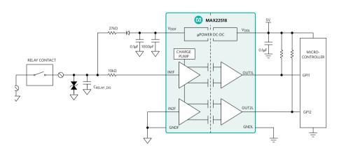
Figure 6. Single-Channel Relay Contact Monitoring with MAX22518
