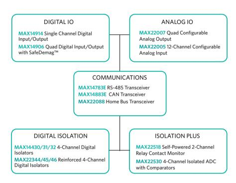
Figure 1. BACS Key Enabling Technologies
