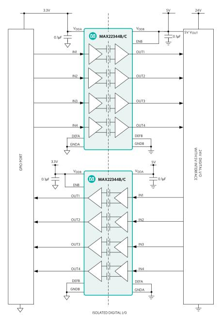
Figure 5. Reinforced Digital Isolators in Digital IO Application
